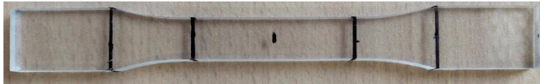
Figure 3 Marked samples for the tensile and fatigue testing
