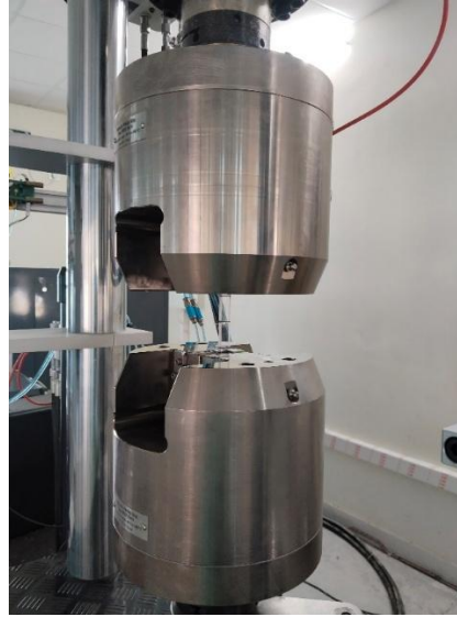
Figure 5 Walter+bai servo-hydraulic UTM testing machine
